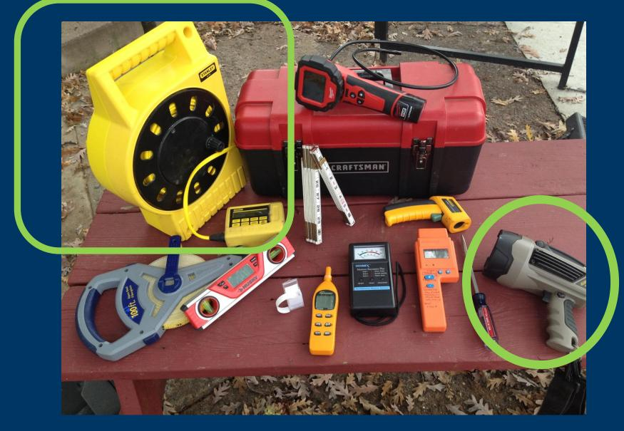
**Moisture Detection** Infrared Camera -Detects changes in temperature -Water will not show up if there is no change in temperature. -Water usually shows up as cooler, BUT not always.
