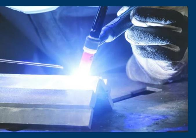
Welding temperatures ranges roughly between 10,000-15,000 degrees Fahrenheit
