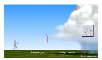
The signal bounces off the particles in the storm and is returned to the receiver.
