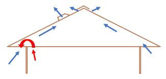
The diagram below shows the same roof with a short in the attic ventilation. For several reasons a soffit vent may be more restrictive in drawing air into an attic than at an adjacent upper vent. The end result is dead air space that may become a problem.
